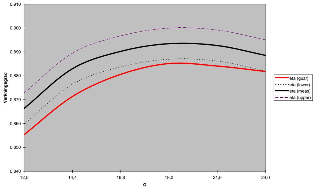
Figure 5. Measured efficiency with inaccuracy bands and guaranteed efficiency
