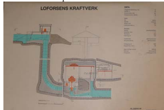
Fig. 1 Placement of the generator
