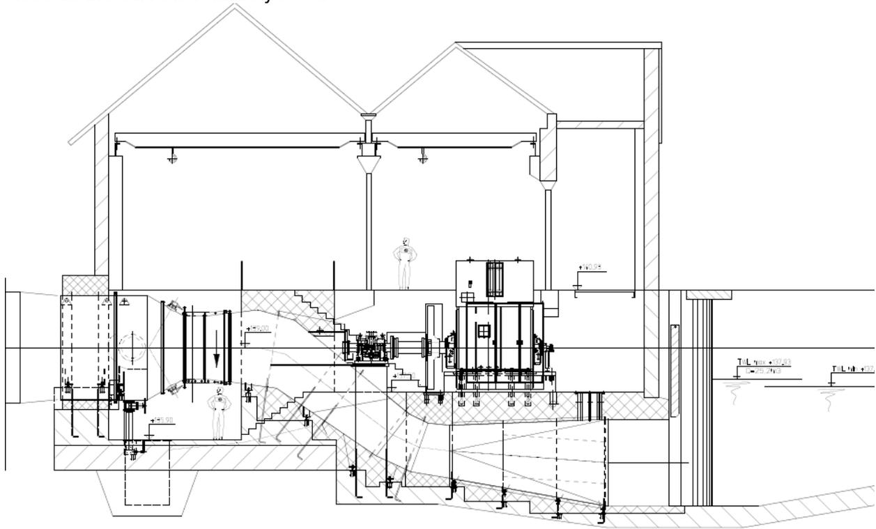
Figure 4 The runner centerline of +139.00 is located above maximum TWL of +137.93
