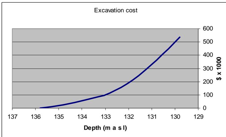
Figure 3 Excavation cost vs depth (Excavation and subsequent construction)
